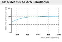
Typical module performance under low irradiance conditions in comparison to STC conditions ( $25 \,^{\circ}$ C,  $1000 \,^{W/m^2}$ ).
